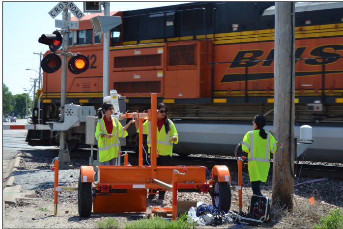
Pictured from left: REU students Gabriela Perales and Cassandra Sias work with Nebraska Transportation Center Ph.D. student, Li Zhao, at a highway rail grade crossing setting up traffic data collection sensors.
