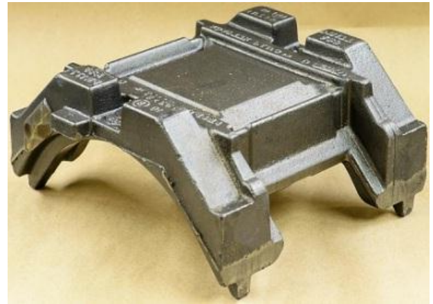
Figure 2: Original Railroad Bearing AdapterPlus™ without Elastomer Pad-Liner
