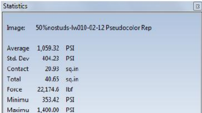
Figure 10: 3D Image Load Pattern and Pressure Statistics at Interface between the Elastomer Pad-Liner and the AdapterPlus™ at ~60% of Full Load
