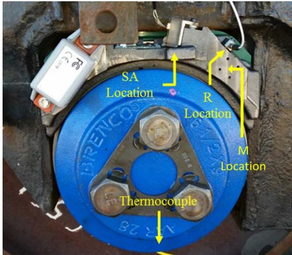
Figure 5. Modified bearing adapter showing sensor locations
