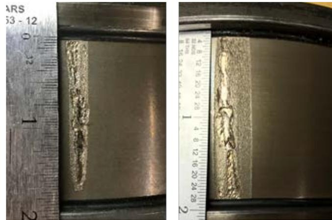
Figure 10. Starting cone spall for Bearing 2 (left); ending cone spall for Bearing 2 (right)
