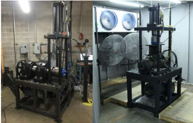
Figure 3. Single Bearing Test Rig (left), Four-Bearing Test Rig (Right)
