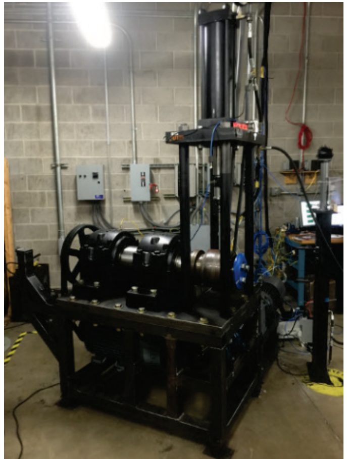
Figure 3. Single Bearing Tester (SBT)
