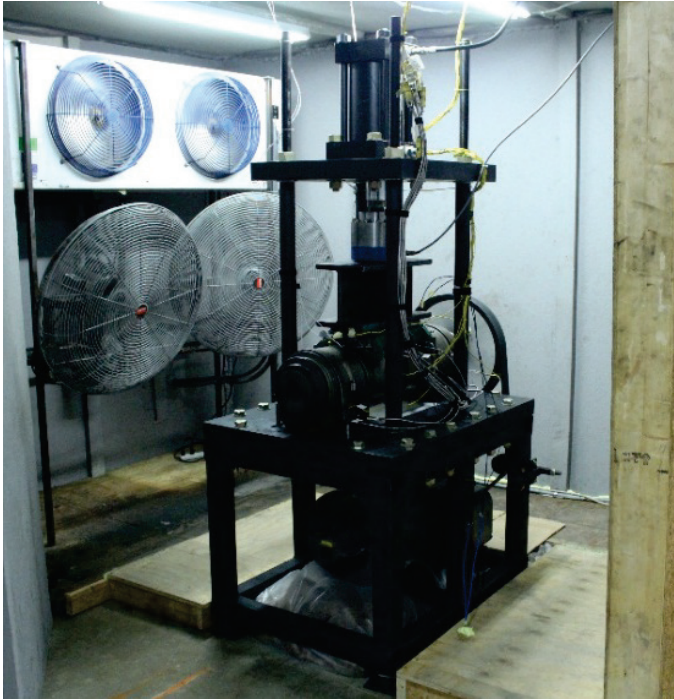
Figure 4. Four Bearing Tester (4BT)
