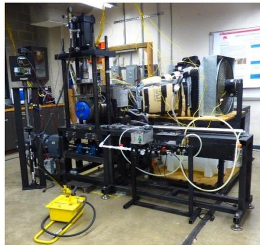
Figure 1. Single Bearing Tester (SBT)
