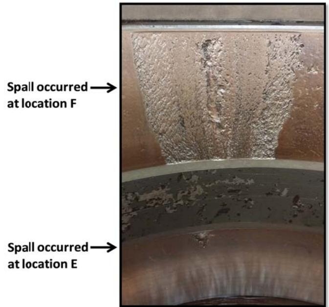
Figure 7: Spalls that developed on the surfaces of the outboard and inboard races (cup) at locations which coincide with the subsurface inclusion sites E and F, respectively.
