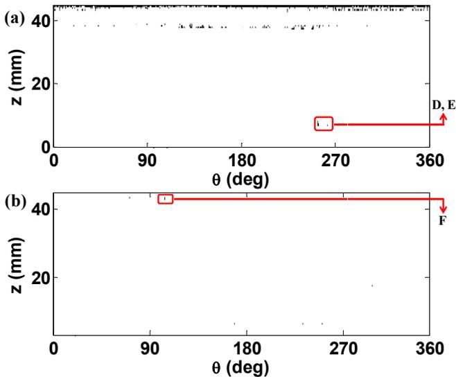
Figure 5: C-Scan image from the cup in the simulated service life testing, (a) two inclusions found using 15 MHz on the outboard race, (b) the only inclusion found using 7.5 MHz on the inboard race.
