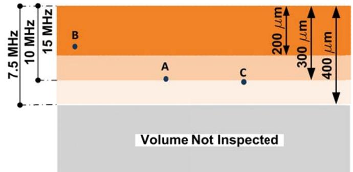
Figure 4: The schematic diagram of presumed locations of inclusions with the relative depths in the sample.
