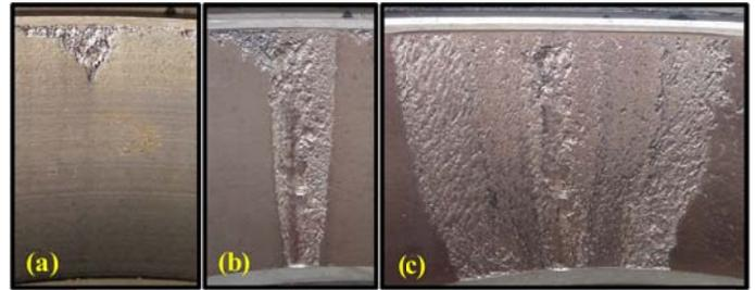
Figure 6: The spall deterioration on an outboard race (cup) at location F, (a) mileage = 51,420 miles, area = 112.709 mm<sup>2</sup>, (b) mileage = 63,678 miles, area = 677.418 mm<sup>2</sup>, and (c) mileage = 77,506 miles, area = 2850.317 mm<sup>2</sup>.
