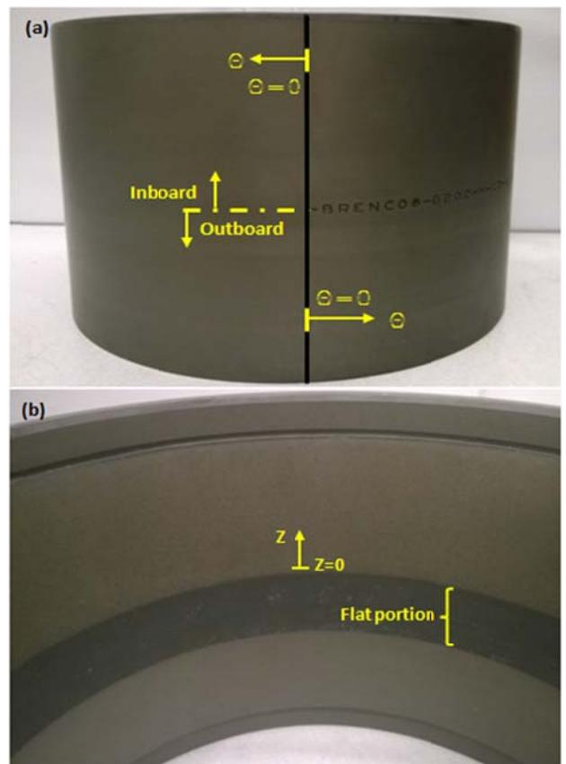
Figure 2: (a) Orientation of the race surfaces (outboard and inboard) and their respective positive  $\theta$  rotations, (b) Origin coordinate of  $z$  and the corresponding positive direction for the both inboard and outboard races.
