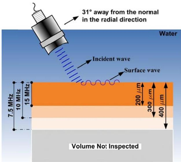
Figure 1: The schematic diagram of an ultrasonic surface wave scan using multiple frequencies on a steel sample.
