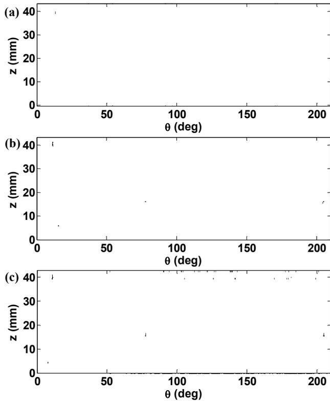
Figure 3: C-Scan images from a cup using three different center frequencies, (a) one inclusion found using 15 MHz, (b) three inclusion found using 10 MHz, (c) three inclusion found using 7.5 MHz.
